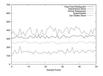
Fig. 2. Illuminance Data over Time at Different Locations
