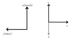
(a) Horizontal plane (b) North meridian plane Fig. 1. The Earth Reference Coordinate System
