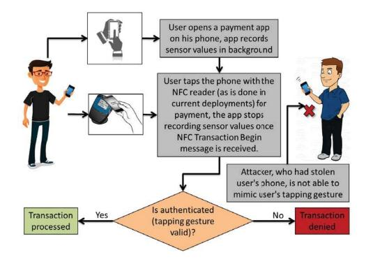
Figure 1: Overview of our system. The user gets authenticated just based on the uniqueness of his tapping gesture, a form of behavioral biometrics. The process is completely transparent to the user – no additional work is needed beyond what is currently done in NFC systems.
