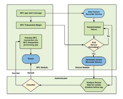
Figure 3: Sensor data collection flowchart.
