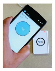
Figure 4: A user tapping an NFC reader at waistflat position. In waist-flat scenario, the NFC reader is kept at the height of 0.75-1 m from the ground and horizontally on the table.
