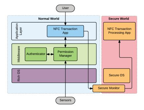
Figure 2: Our System Architecture: Control Flow
