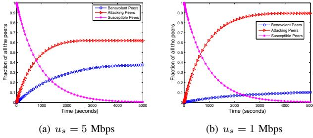
Fig. 3. Impact of server upload bandwidth: when the server bandwidth is high, the long-run fraction of attacking peers decreases greatly.
