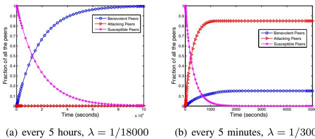
Fig. 4. Impact of patch request rate (a) Every 5 hours: when the request rate is very low, all the requests can be handled by the server and there is no increase in the number of attacking peers. (b) Every 5 minutes: when increasing the request rate, the long-run fraction of attacking peers also increases.
