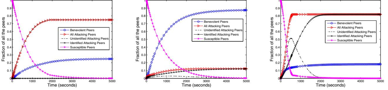
(a) No honeypots, scanning rate  $\beta = 0.001$  (b) 80 honeypots are used, scanning rate  $\beta = 0.001$  (c) 80 honeypots are used, scanning rate  $\beta = 0.01$
