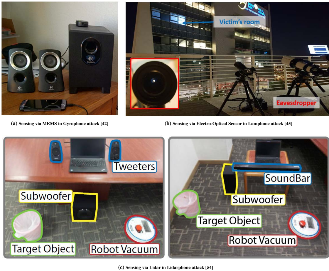
Figure 4: Images of experiments conducted in three vibration-based side-channel attack papers that eavesdrop speech via different sensor methodologies.
