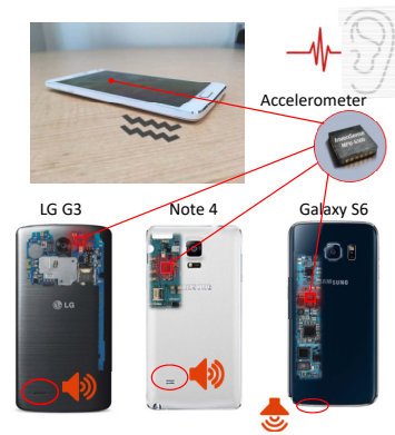
Figure 10: The speaker and the sensor positions on the smartphones of different vendors.
