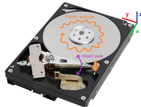
Figure 7: Force diagram showing the natural vibrations internal to HDDs.
