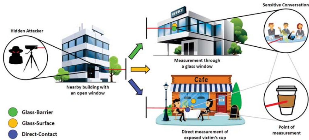
Figure 1: A malicious attacker can take advantage of three potential attack scenarios to eavesdrop on speech. Green: an attacker can direct their laser through the window of a building and focus on a cup that is near the speech source ( Glass-Barrier ). Yellow: an attacker can focus their laser on the surface of a nearby window ( Glass-Surface ). Blue: an attacker can focus their laser directly onto an exposed cup without passing the laser through a glass barrier ( Direct-Contact ).
