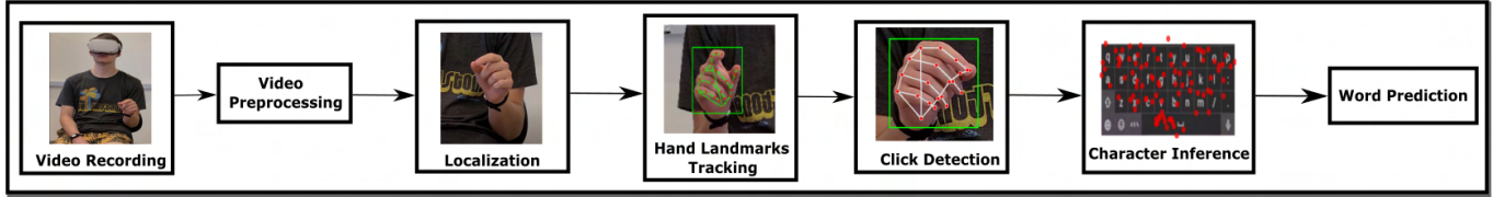
Figure 3: Figure shows the steps involved in the execution of the Hidden Reality attack model. An adversary captures the video footage of a targeted user while the user is performing typing operation on their virtual screen. Region of interest is obtained by localizing the typing hand and tracking the hand landmarks points on the preprocessed video. By mapping the tracked hand pixel location coordinates obtained in the click detection step onto the known keyboard geometry, the typed text gets inferred.
